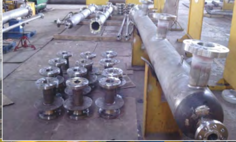
Compressor Piping Spools
