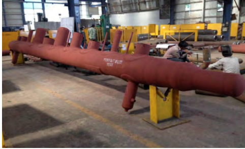
Main Stream Piping Spool
