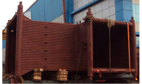
CFBC, Fully Assembly Cross Over Duct
