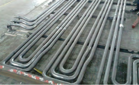
Super Heater Coils
