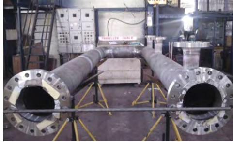
Compressor Piping Spool
