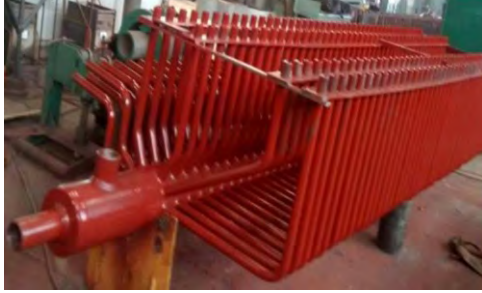
Primary Super Heater Header
