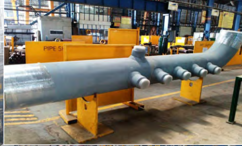
Pre-Fabricated Piping Spool
