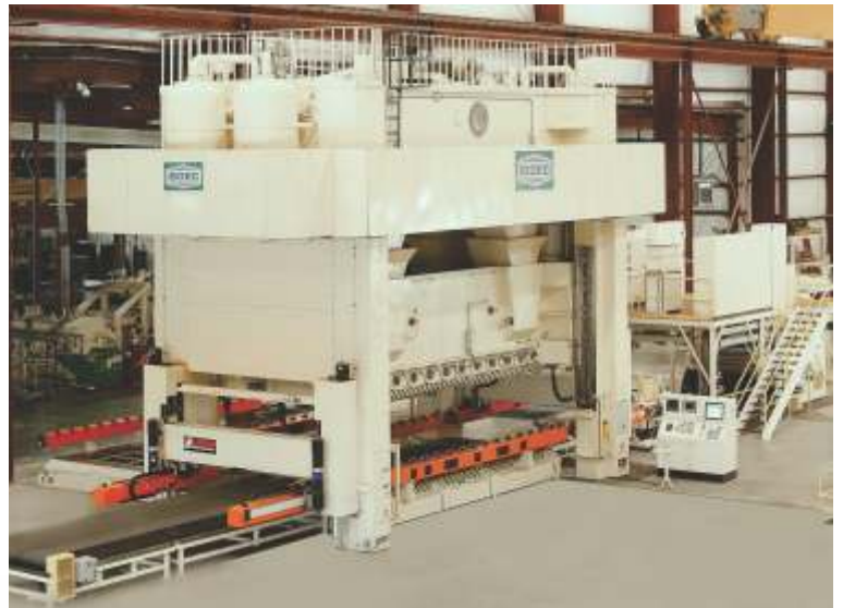
20000 kN Mechanical Transfer Press Big Rapids Products, Kentucky, USA Bolster Size 7600 mm x 2800 mm, 3-Axis Servo Transfer System
