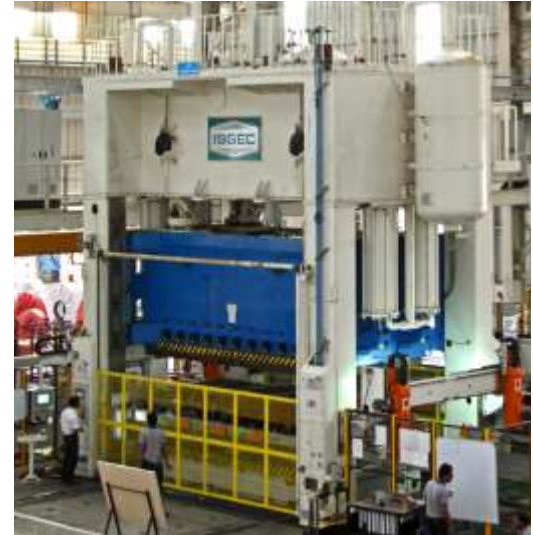
12500kN Transfer Press with bolster size 5000mm x 2500mm & 15-30 SPM
