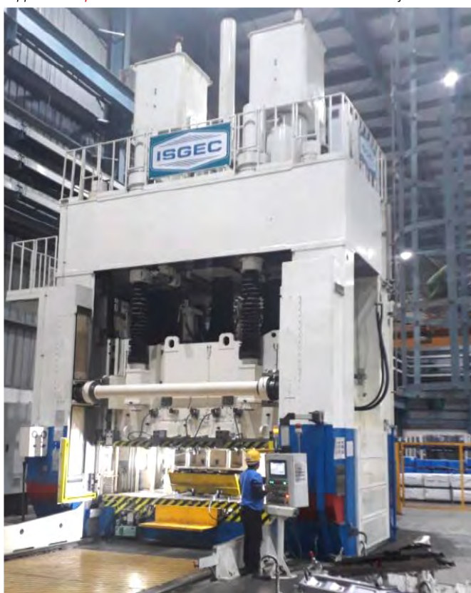
1200 T Tryout cum 300 T Die Spotting Press with 180 deg Slide Tilting feature supplied to Japanese Auto Tier-1 for their JV in India for Suzuki Project
