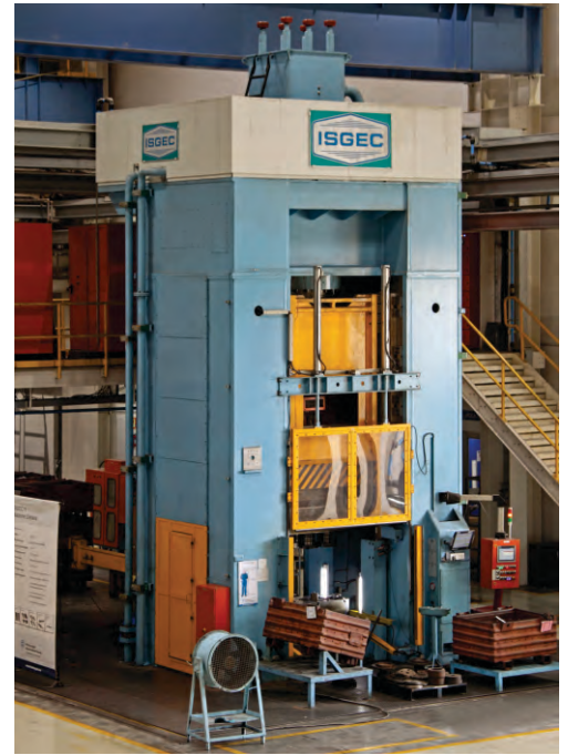
1600T Hydraulic Press for manufacturing Cold Forged Automobile Transmission Components in India
