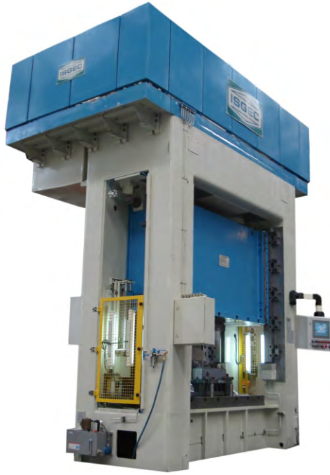
315T Hydraulic Press supplied to a customer in Romania
