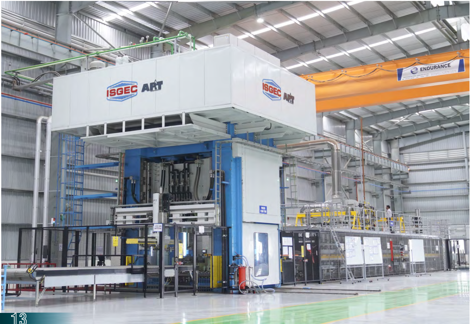
1200T Hydraulic Hot Forming Press at Tier-1 automobile supplier in India
