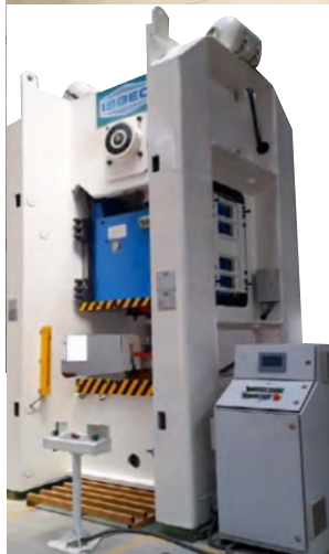
250 T MAX 1 Monolithic Frame Single Crank Press supplied to Auto Tier-2 in India. MAX 1 Models are available from 200 T to 400 T
