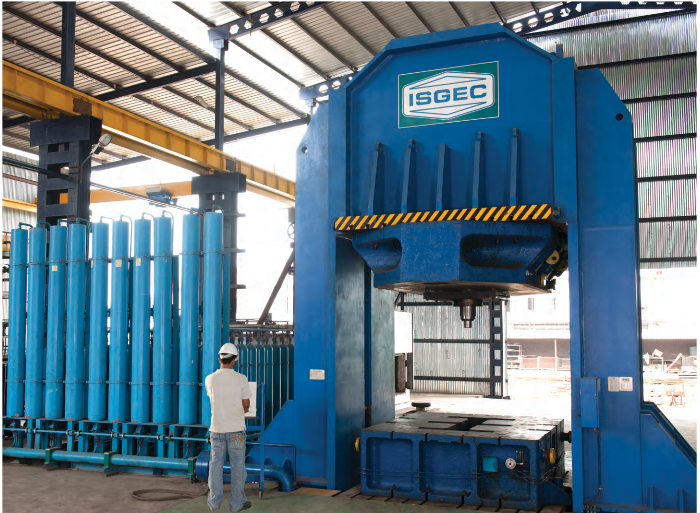
12500T Hydraulic Press with large Accumulator Bank is being used for Hot & Cold Forming of High Tensile Steel Plates for Defense & Aerospace Applications
