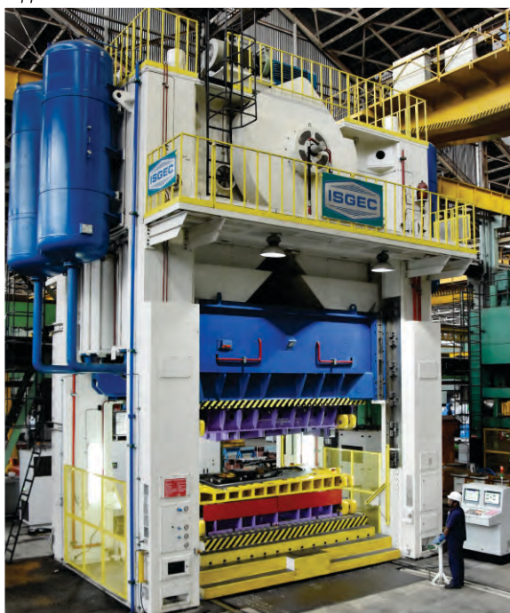
2000 T Mechanical Tryout Press with full force Micro Inching supplied to Tata Motors
