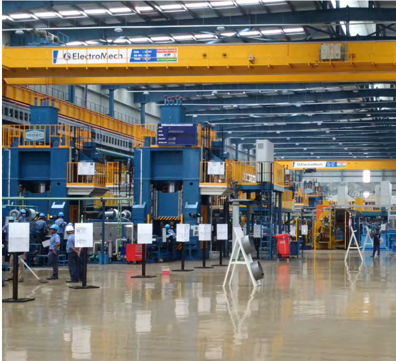
Range of hydraulic presses supplied to a major Tier-1 automobile supplier in India for manufacturing wheels
