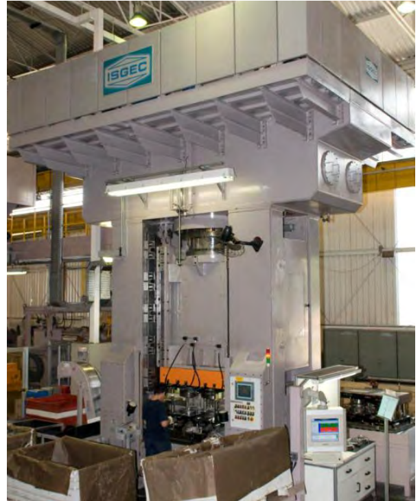
1500T Hi-speed Hydraulic Press supplied to a German MNC in Brazil for manufacturing Clutch Components. Similar supplies made to their plants in South Africa & India
