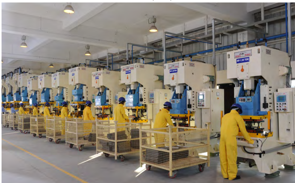
Battery of Gap Frame Presses supplied to Automotive Tier1 Industry in India. Gap Frame Presses GZ/GL series are available from 40T to 400 T. Link Motion and Medium Speed options are also available
