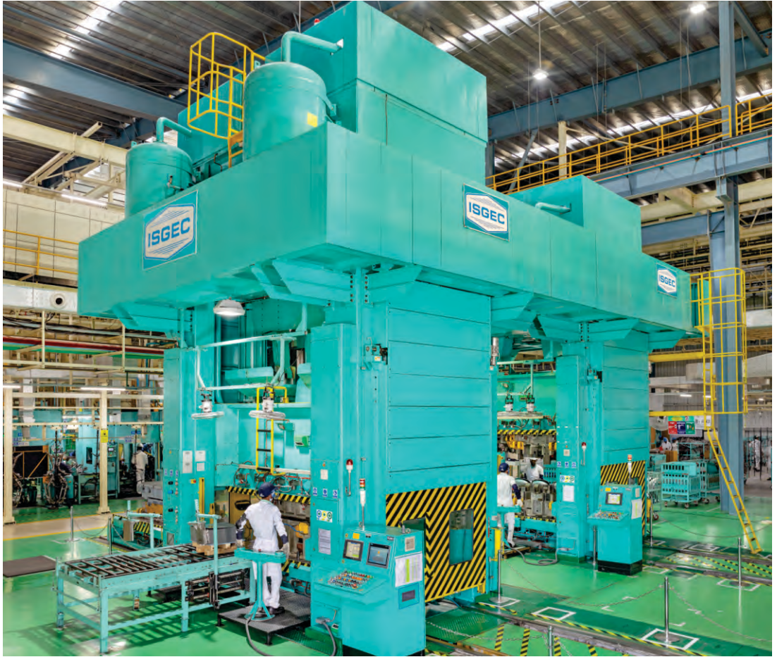
630 T Link Drive & 400 T Eccentric Gear Drive Tandem Line supplied to Japanese OEM in India for manufacturing of Two Wheeler Components
