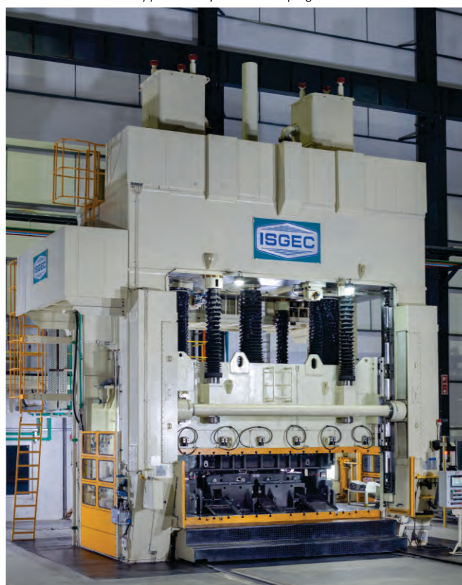
1000 T Tryout cum 300 T Die Spotting Press supplied to Japanese Stamping Dies manufacturer in India
