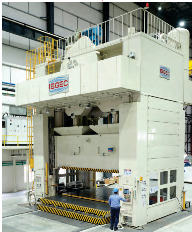
1500T Mechanical Tryout Press Supplied to a Japanese MNC.
