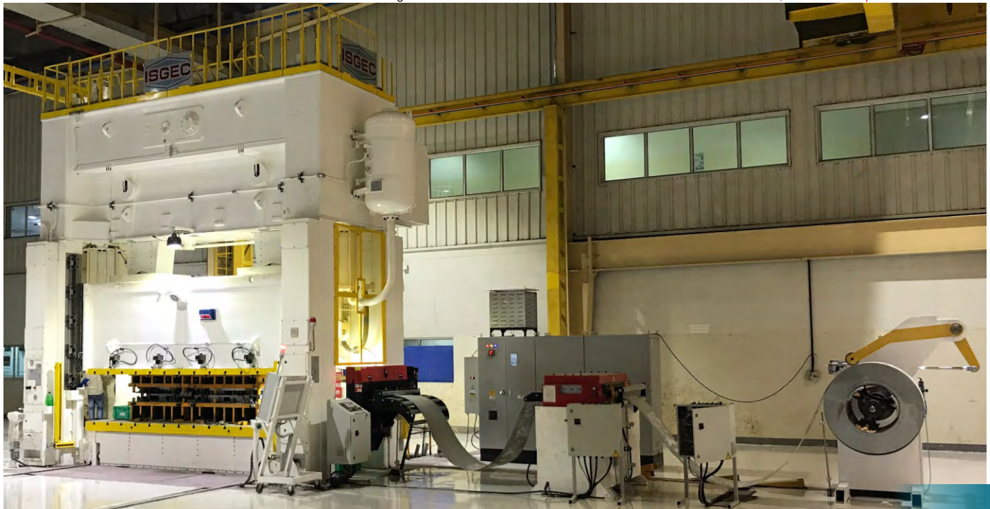
400 T Progressive Die Mechanical Press with Bed Size 4000 mm x 1500 mm, installed at Japanese OEM in India
