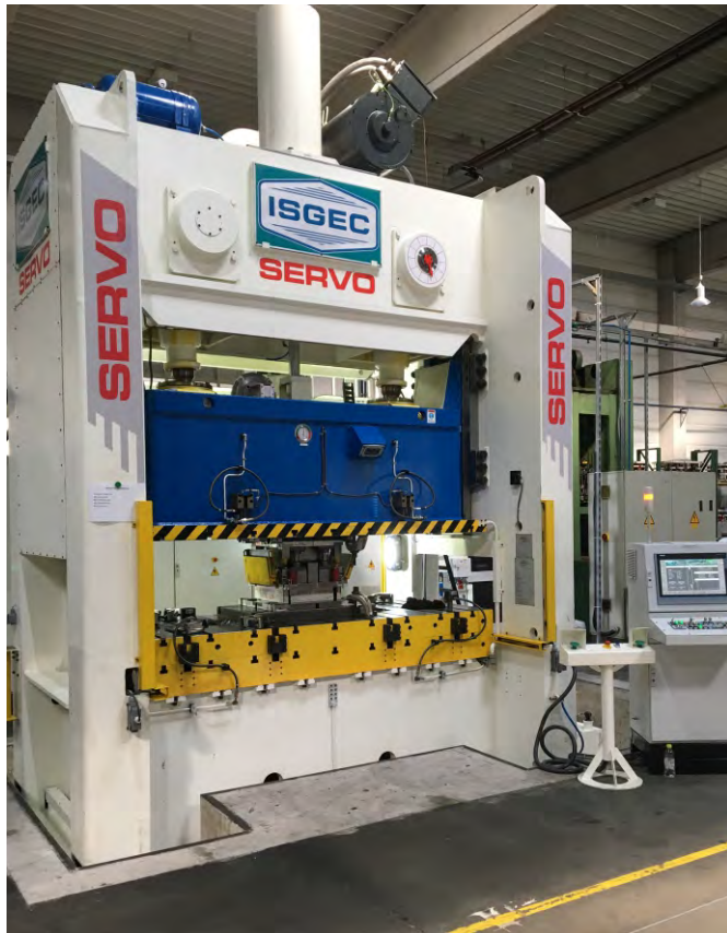
630T & 400T Straight Sided Servo Mechanical Press supplied to a customer in Hungary
