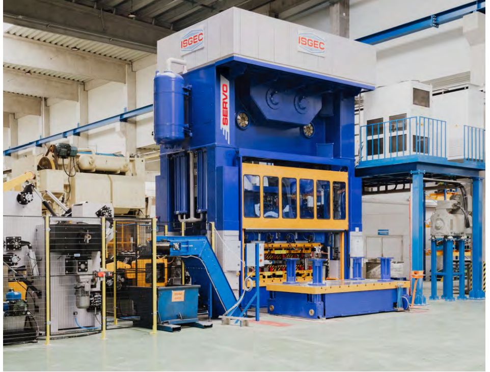
630 T Servo Mechanical Press with Bolster Size 3400 mm x 1600 mm and 3-50 spm installed in Slovakia for Progressive Application
