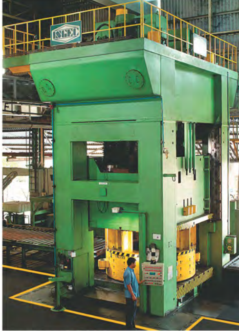
Installed at Wheels India, a TVS Group Company , this 20000 kN Hydraulic Press, having a bed size of 3000 mm x 3000 mm, is used for Hot Forming of Earth Mover Wheels for Caterpillar and Komatsu.
