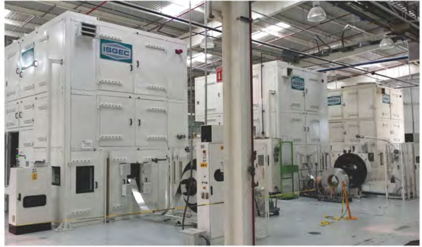
A line of 2000 kN High Speed Presses installed in Mexico to produce Automotive Heat exchanger Plates @ 200 spm.
