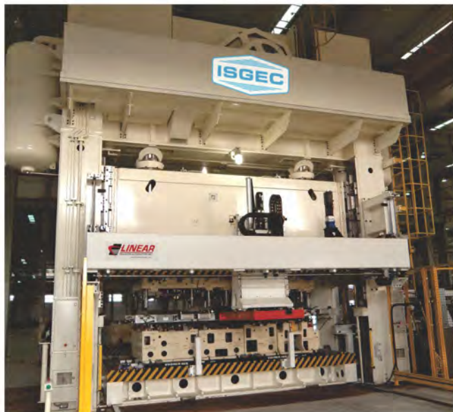
12000 kN Transfer Press supplied to a MNC Car Seat producer for their plant in China . Bolster Size 5500 mm x 2500 mm, equipped with 3 Axis Electronic Servo Transfer System & Destacker.
