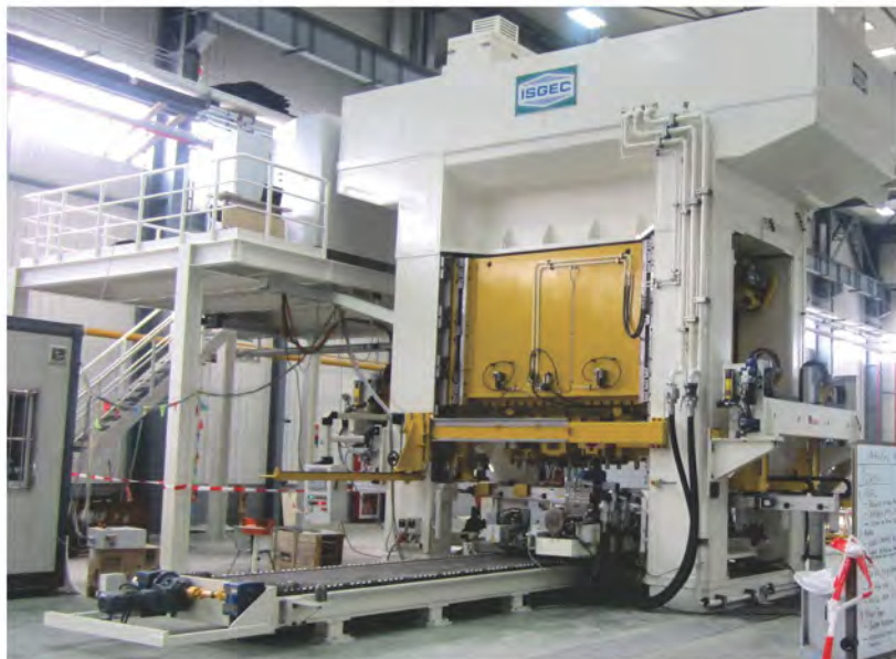
8000 kN Hydraulic Transfer Press with Parallelism Control System, Supplied to Benteler Group for their plant in Shanghai, China
