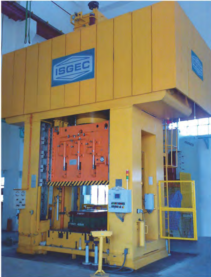
This 7500 kN Hydraulic Press has been supplied to Franke, Switzerland, for their Aurangabad Plant in India. Franke is market leader in the manufacture of Kitchen Sinks. The first Hydraulic Press of 630 T was supplied in the year 2000, followed by a second Press in 2009.
