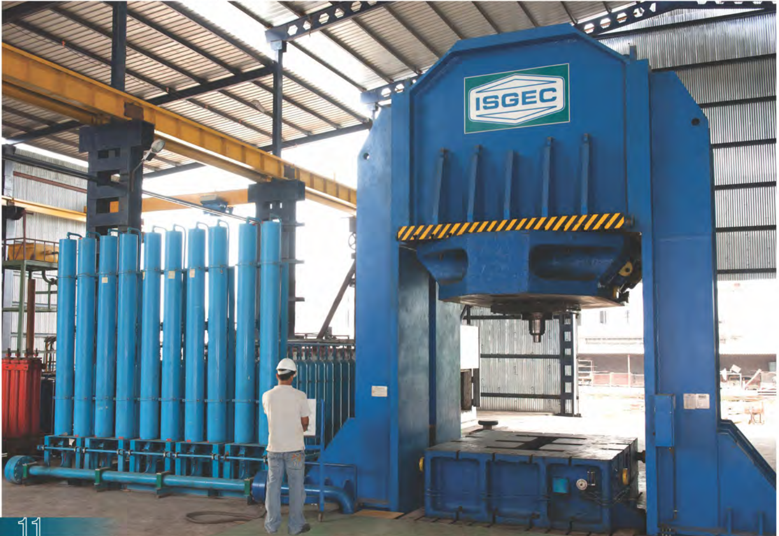
125000 kN Hydraulic Press with large Accumulator Bank is being used for Hot & Cold Forming of High Tensile Steel Plates for Defence & Aerospace Applications
