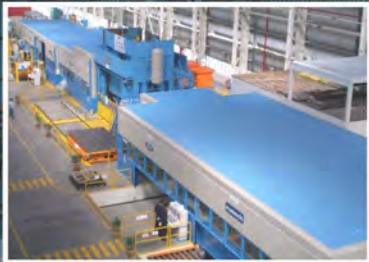
The above picture shows 5000 kN Blanking Press supplied to Ford Motors, India .
