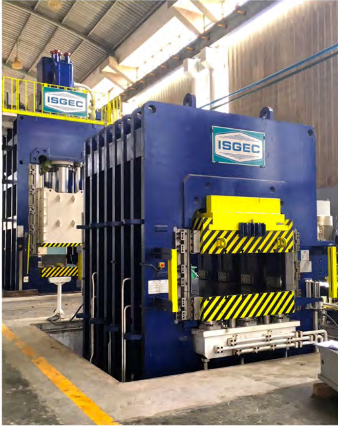
7000T and 2000T Hydraulic Presses supplied to manufacture Heat Exchanger Plates for High Capacity Industrial Heat Exchangers
