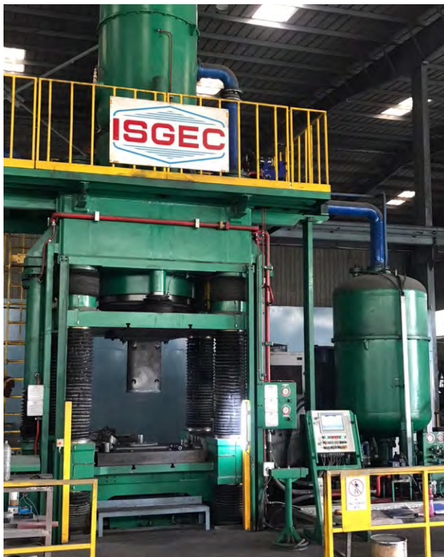
2500T Press for Refractory Brick, Nozzle and Slide Gate Manufacturing
