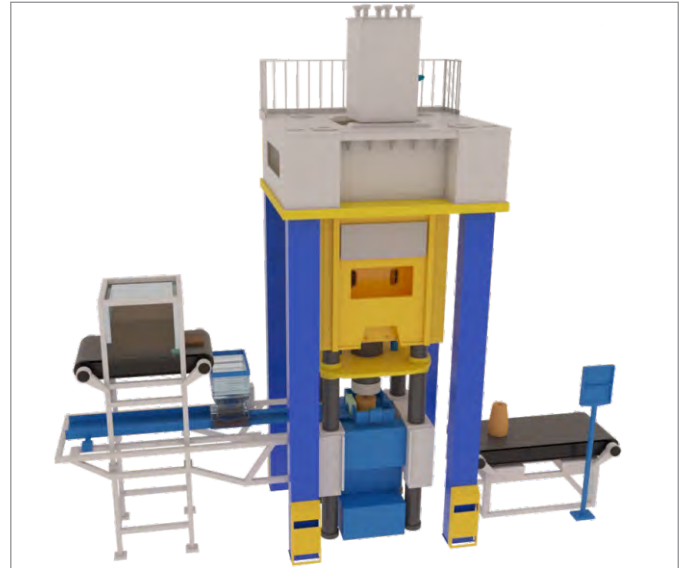
Nozzle manufacturing with Automatic Mould Filling and Unloading
